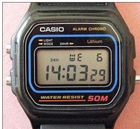
Fig. 5. A Casio Alarm Chrono digital watch with liquid crystal display (LCD). It displays a small number of individual digits or fixed symbols as in digital watches and pocket calculators (1).
