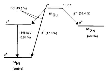
Figure 2. Decay scheme of Cu-64 with intensities of emitted radiations (after Ref. [11]).
