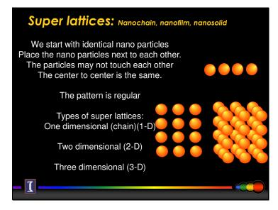
Figure 14. Super Lattices: Nanochain, Nanofilm, Nanosolid.
