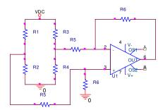
Figure 4. Sensor Integration Circuit.
