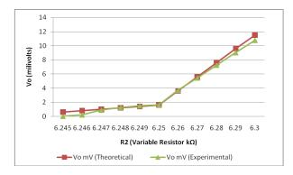
Figure 6. Comparative study between Theoretical, Simulation and Experimantal results on output voltage of Integration of Sensor and Transduction Stage.
