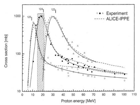
Figure 3. Excitation functions of (p,xn) reactions on Te-125 leading to the formation of the radionuclides I-125, I-124 and I-123. The solid lines are eye-guides through experimental data. The broken lines show the results of nuclear model calculations using the code ALICE-IPPE. The shaded area gives a suitable energy range for the production of I-124 (after Ref. [12]).
