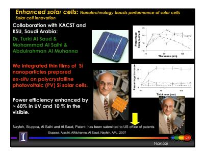
Figure 22. Enhanced Solar Cell: Nanotechnology Boosts Performance of Solar Cells.
