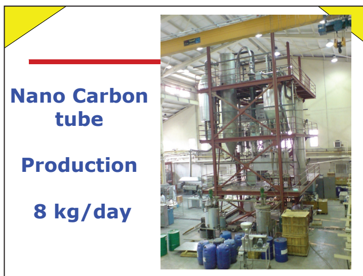
Figure 25. Nano Carbon Tube Production 8kg/ day.
